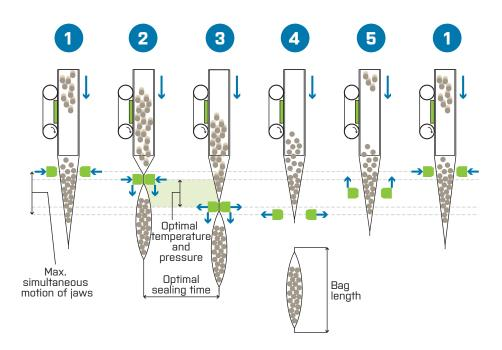
The special power sealing mechanism drives the cross sealing jaws, which exert the necessary force to achieve perfect seals with a wide range of films.
